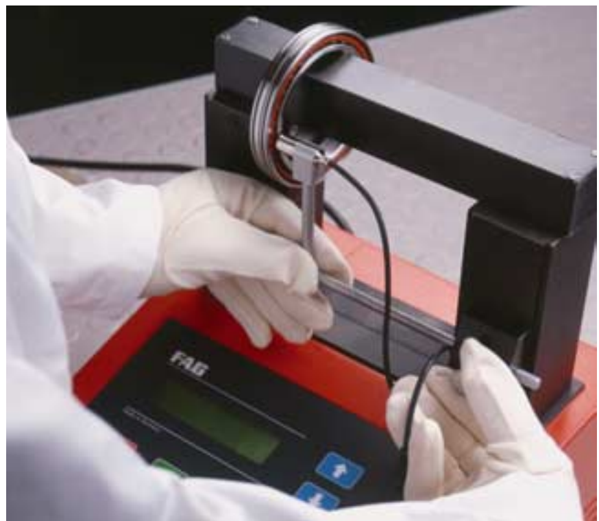
40: Mounting using an induction heating device
